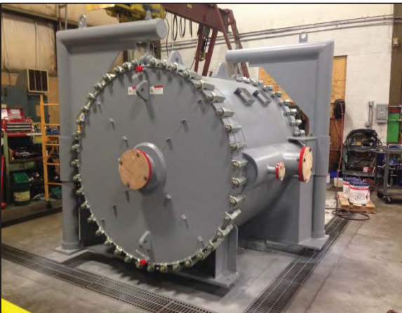
OIL & GAS: Produced Water Cooler; Carbon Steel
