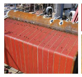
THE RENTECH BOILER SYSTEMS HEADERED MEMBRANE FRONT AND REAR WALLS ELIMINATE THE PROBLEMS ASSOCIATED WITH OTHER DESIGNS
